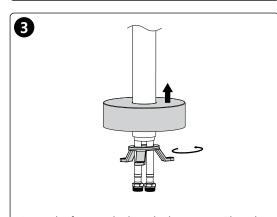
Insert the faucet tube into the base cover. Thread the tube onto the mounting tripod.
