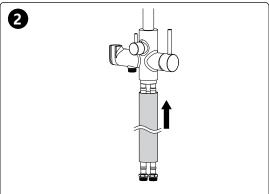
Insert faucet body assembly onto the faucet tube from the top and hand tighen it.Make sure the flexible water supply lines go through the tube smoothly.
