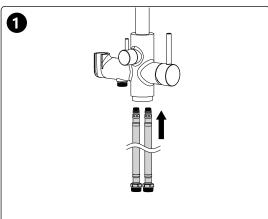
Hand tighen the hot and cold flexible water supply line onto faucet body.
