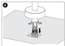
Locate the faucet assembly onto the rough valves from floor, and secure the connection of inlet supply lines to the valves. **DO NOT** reverse the Hot and Cold supply.
