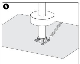
Using the mounting piece as a template, mark the positions of the screw holes.
