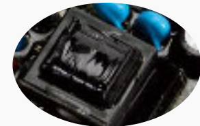
Gluing treatment, waterproof upgrade
