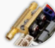
Thyristor water cooling
